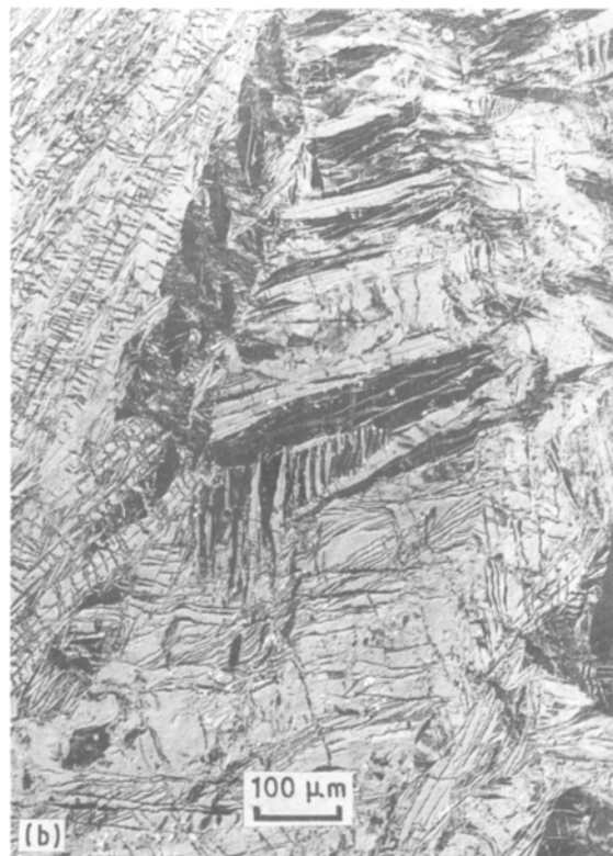
Figure 4 Microstructure of the transformed DSC specimen. (a) Undeformed, (b) cold-rolled at T = -196\text{ }^{\circ}\text{C} .
